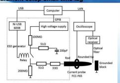
Current and spark two paths measurement setup
