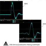
· Introduction of a ferrite to meet previous specs to meet FWHM requirements introduces significant ringing when viewed with a high BW scope (not seen at 1 GHz)
