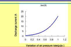
Discharge current in surface process decrease rapidly with gas pressure increase
